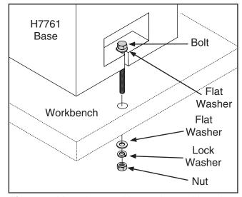
Figure 3. Mounting machine to the workbench.
